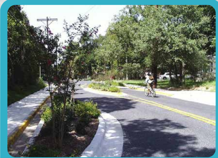
Lane shift and chicanes to slow traffic down and increase driver attentiveness; chicanes can be planted to improve visual appeal and reinforce neighborhood character
