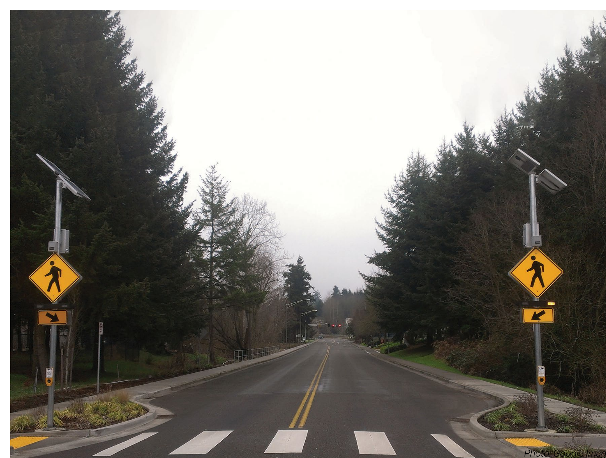
PEDESTRIAN CROSSING, REFUGE AREA, AND CURB EXTENSIONS
